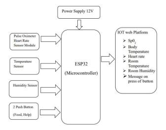
Fig 2 : Block diagram of Remote Intensive Care Unit Monitoring and Communication
